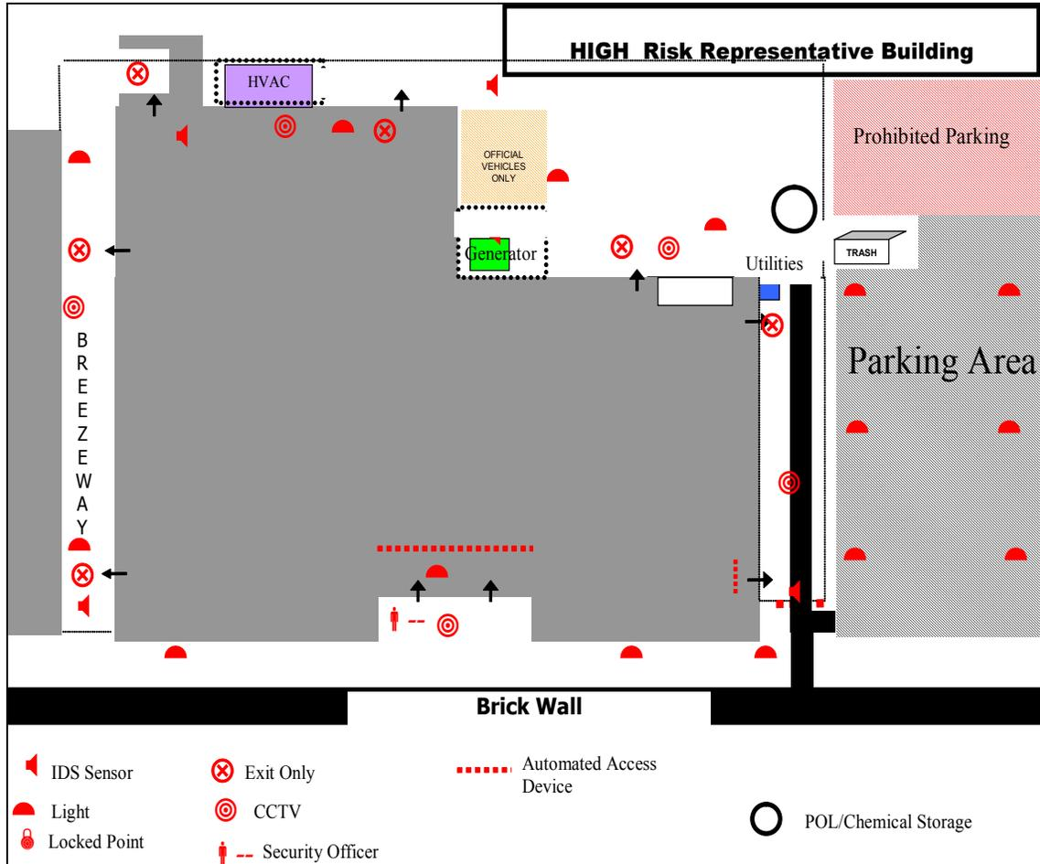
This diagram shows a high-risk building depicting physical security tools and technologies. The intent is to show how these systems should be used to complement each other and to provide a layered and overlapping security approach to facility protection.
